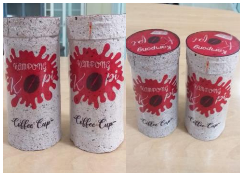
Figure 4. Coffee packaging products from recycled paper made from coffee leather and used paper waste.
