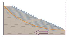
Figure 29. The results of soil nailing reinforcement modeling on slopes using GEO5 with earthquake loads at STA 444+350/450.
