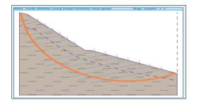
Figure 17. Slope reinforcement modeling results with soil nailing on GEO5 without earthquake loads at STA 436+1/2.
