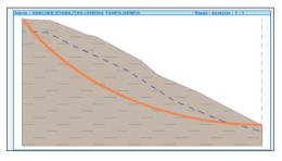
Figure 23. Modeling results using GEO5 for existing conditions without earthquake loads at 444+350/450.
