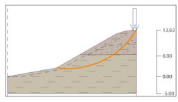
Figure 33. Modeling results using GEO5 for existing conditions without earthquake loads at 490+870.
