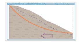
Figure 25. Modeling results using GEO5 for existing conditions with earthquake loads at STA 444+350/450.
