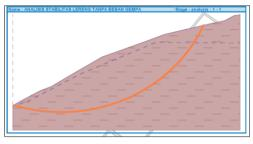
Figure 3. Modeling results using GEO5 for existing conditions without earthquake loads at STA 435+650/850.
