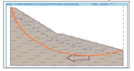
Figure 19. The results of soil nailing reinforcement modeling on slopes using GEO5 with earthquake loads at STA 436+1/2.
