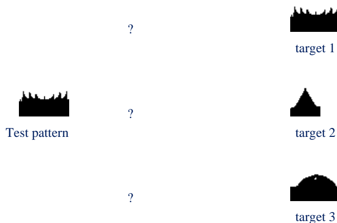
Figure 6 Illustration of Pattern Recognition Using Template Matching
