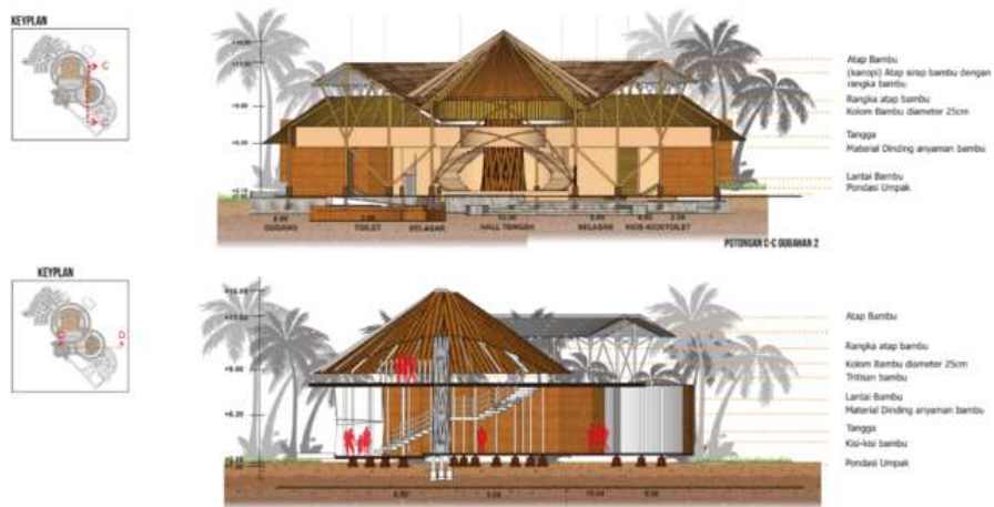
Figure 9. Building section Source : Researcher's analysis, 2022
