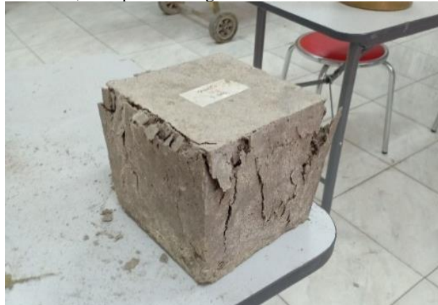
Figure 6. Crack Pattern of Concrete in the 25% Mixture.
