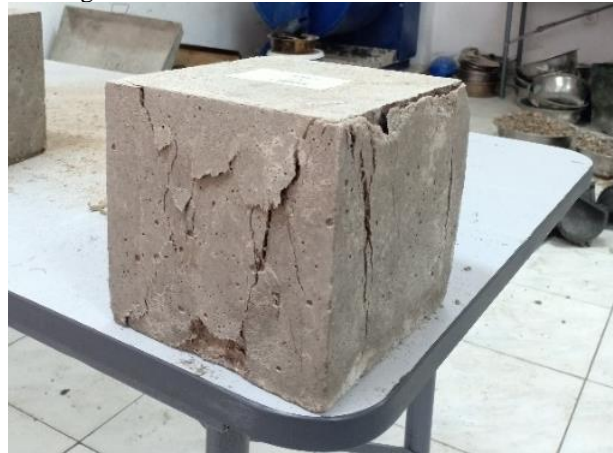
Figure 5. Crack Pattern of Concrete in the 0% Mixture.
