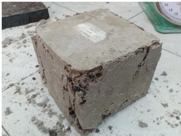
Figure 7. Crack Pattern of Concrete in the 60% Mixture.
