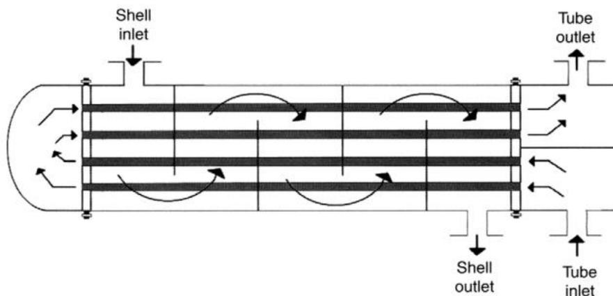
Figure 1 Schematic Illustration of a Shell-and-Tube Heat Exchanger [4]
