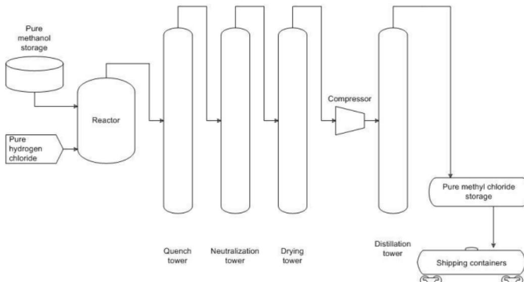
**Figure 2 Scheme of The Methyl Chloride Production [5]**
