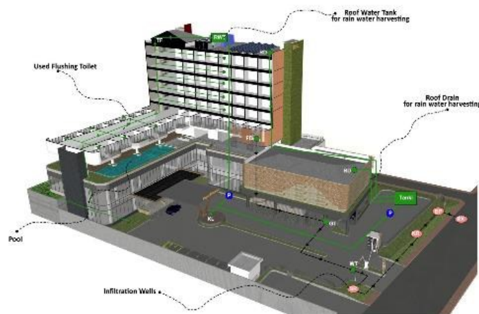
Figure 12 Schematic Design of Rainwater Utilization
