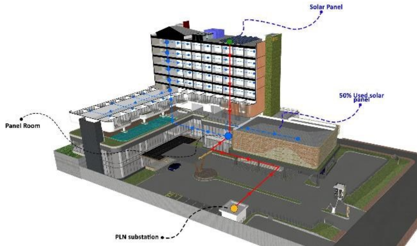
Figure 16 Schematic Design of Electrical Energy Supply
