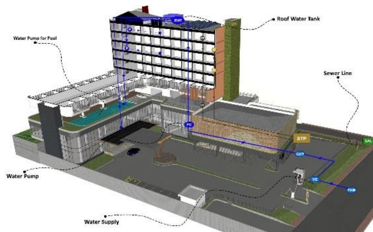
Figure 14 Schematic Design of Clean Water Supply System
