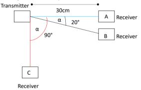
Figure 7. Schematic of beam angle test
