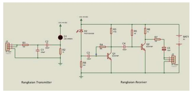
Figure 3. Schematic of the transmitter and receiver circuit on Visible Light Communication
