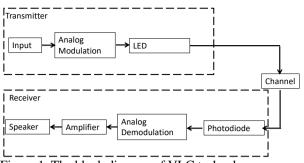
Figure 1. The block diagram of VLC technology
