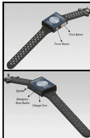
Figure 3. CAD of Smart Exercise Band
